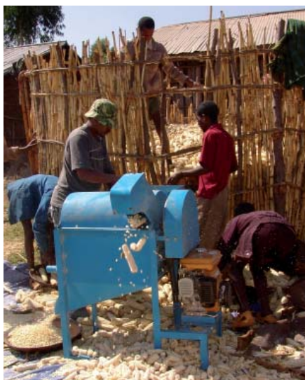
A new portable maize sheller, developed by Selam Awassa in Addis Ababa, Ethiopia, can shell 60% more grain per hour than previous models.
