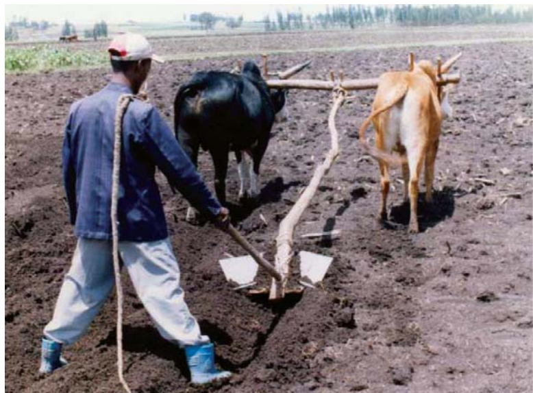
The improved Broad Bed Maker (BBM) in action on Ethiopian vertisol soils. The BBM allows for earlier planting of wheat and, when used in combination with other recommended agronomic practices, leads to significantly higher yields.
