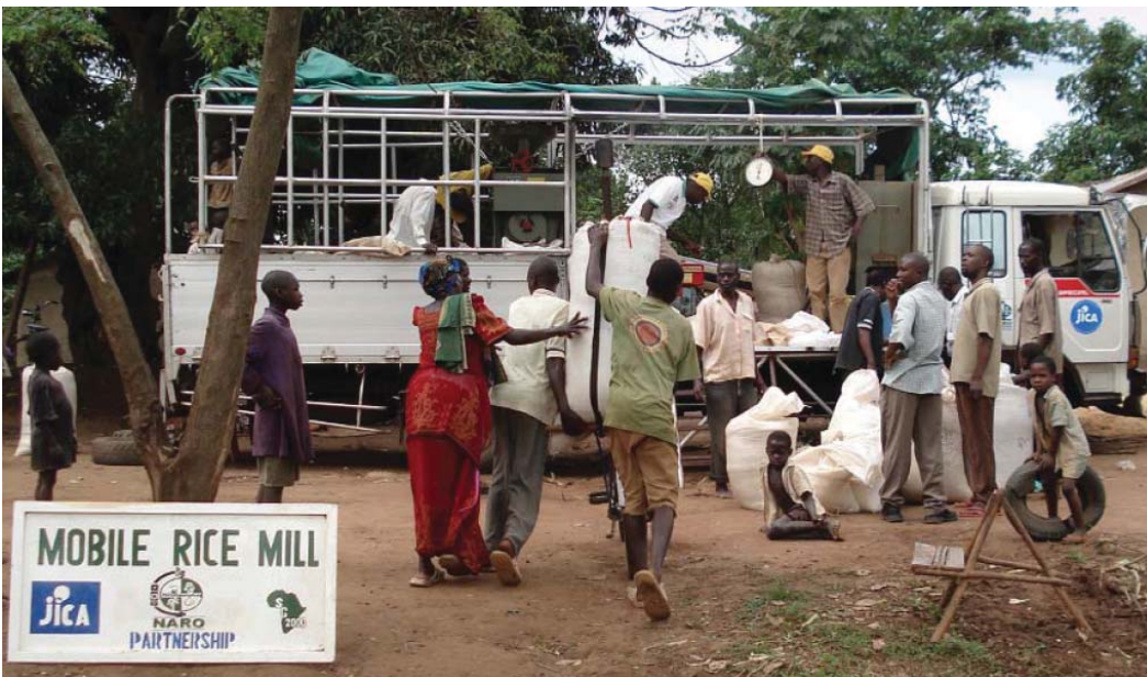
The Japan International Cooperation Agency (JICA) has been testing a new mobile rice mill in Uganda. Some of the country's new rice-growing areas lack access to milling services, so a small mill has been mounted on a truck to bring milling services to more remote farmers.
