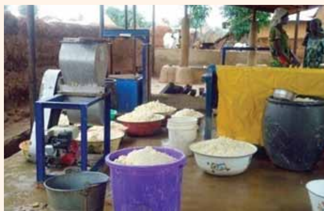
Garri processing enterprise in Nigeria. Following a needs assessment in Adamawa State, SAA provided a women's group with garri processing machinery and the relevant training on operation and business management. The group now processes 270-350kg of cassava per hour, compared to the 10-15kg per hour previously produced using traditional methods.
