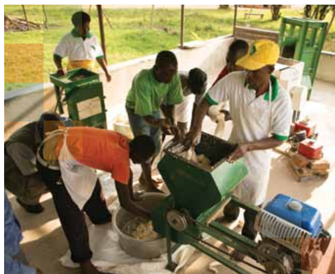
Grating cassava for garri making (cassava agroprocessing) in Pallisa
